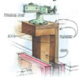
A picture-framing vise, or miter clamp, has screw holes on the bottom for attaching to a workbench. But for occasional framing it can get in the way of other benchwork. A solution is to mount it on a wooden base that can be readily clamped and unclamped in your bench vise. The base can be of scrap wood, and made up so that the framing vise will be about chest high for comfortable working.
